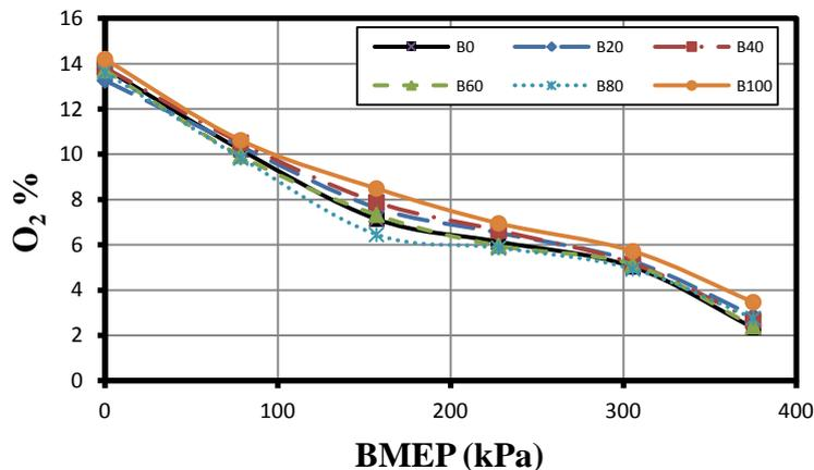
Figure 9: O<sub>2</sub> gas emissions for the tested fuels versus BMEP.
