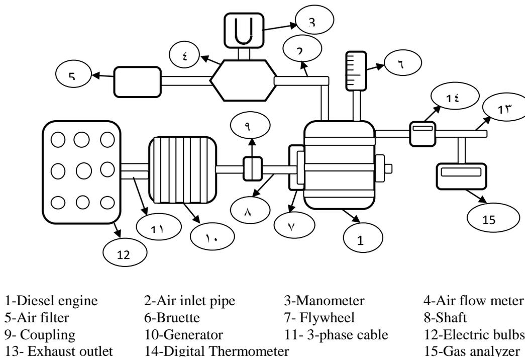
Fig.1: Test engine set-up.
