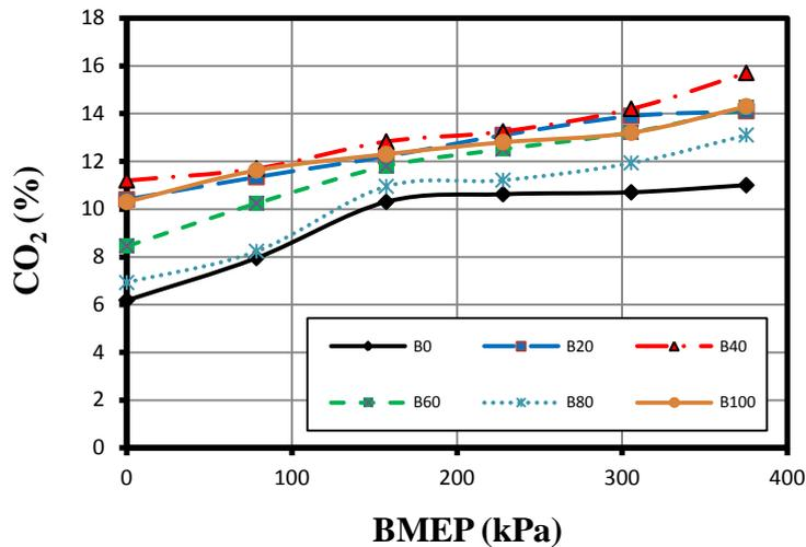
Fig.7: CO<sub>2</sub> gas emissions for tested fuels versus the BMEP.
