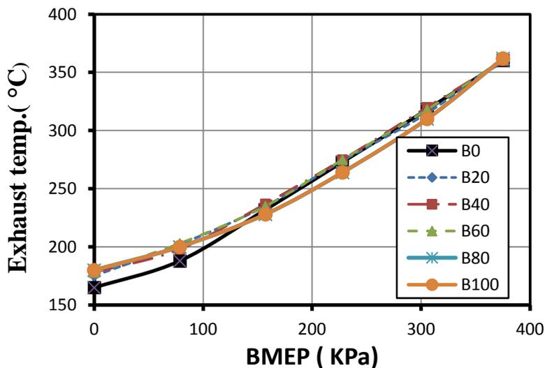
Fig. 5: Exhaust gas temperature for the tested fuel versus BMEP.
