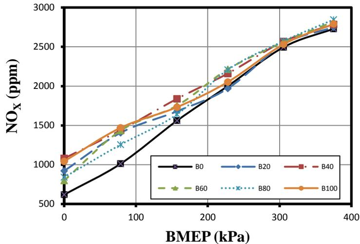
Fig. 8: NO<sub>x</sub> emissions for the tested fuels versus the BMEP.
