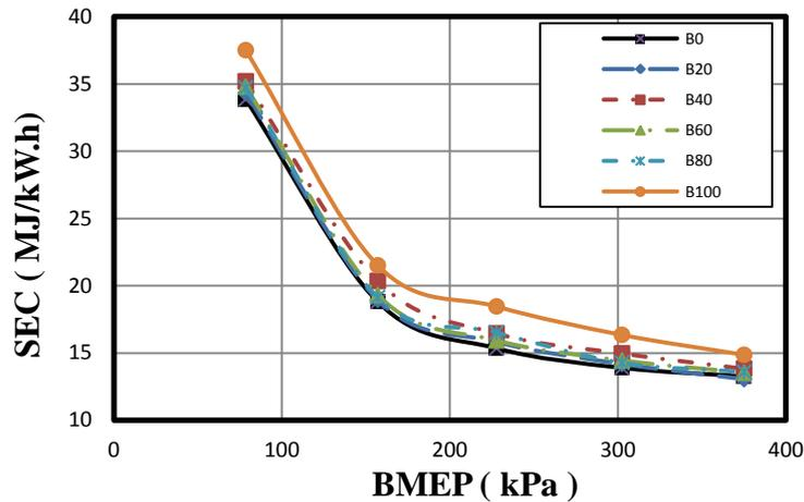
Fig.4: Specific energy consumption for tested fuels versus BMEP.
