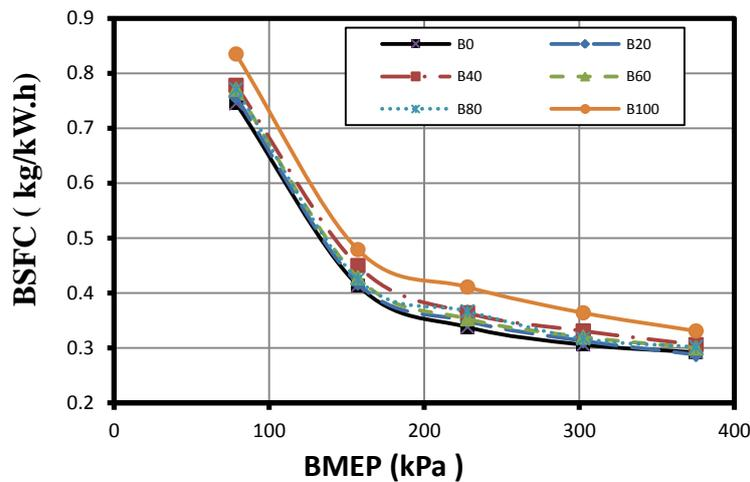
Fig.3: BSFC values for the tested fuels versus BMEP.
