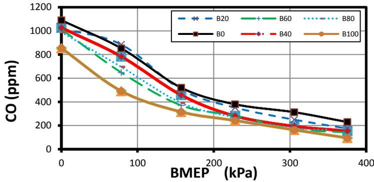
Fig. 6: CO gas emissions for the tested fuels versus the BMEP.
