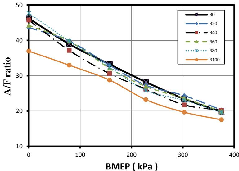
Fig.2: A/F ratios versus BMEP values for different fuel blends.
