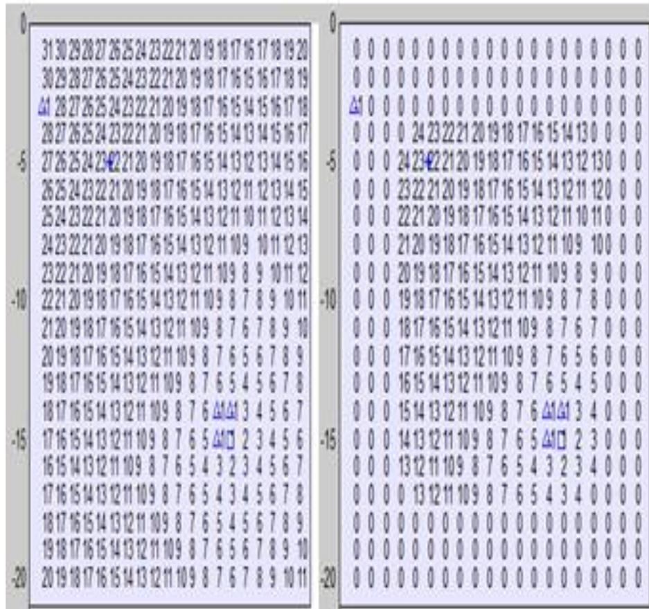
(a) Wave front algorithm expanded. (b) Modified wave front algorithm expanded
