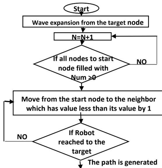
Fig. 3, Flow chart of Modified wave front algorithm
