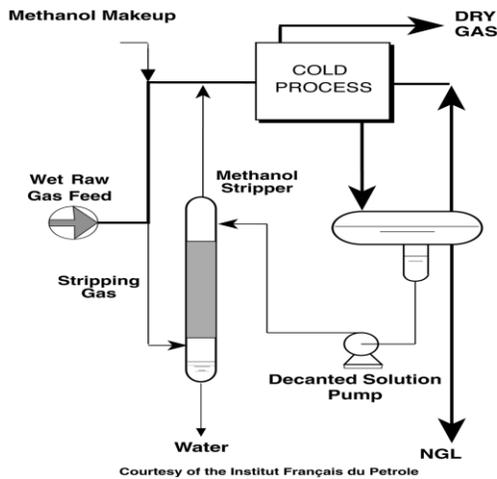
Figure-4 Basic Flow scheme for dehydration by expansion refrigeration
