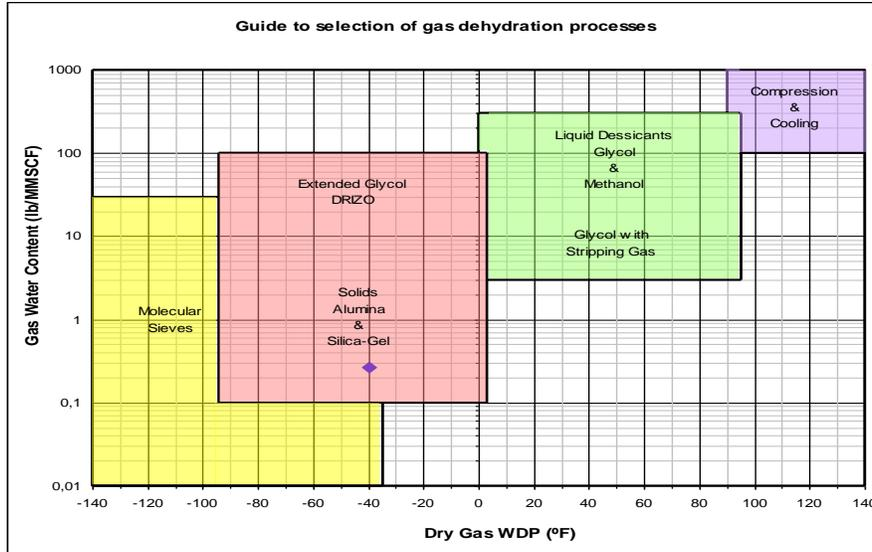
**Figur-6 Gas dehydration technology selection chart**
