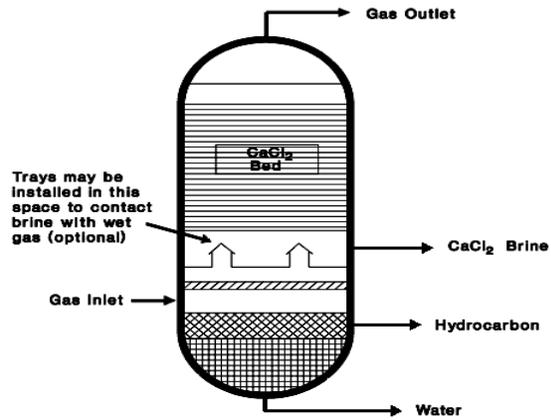
Figure -5 Basic Flow scheme for dehydration by  $\text{CaCl}_2$
