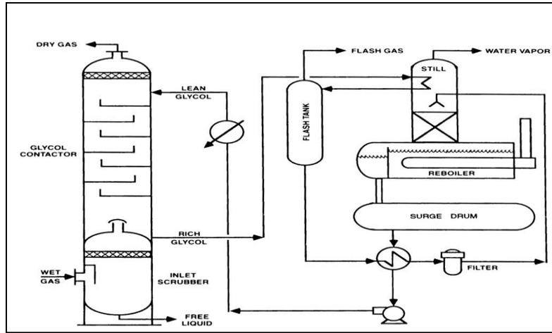
Figure -1 Basic Flow scheme for Glycol Dehydration
