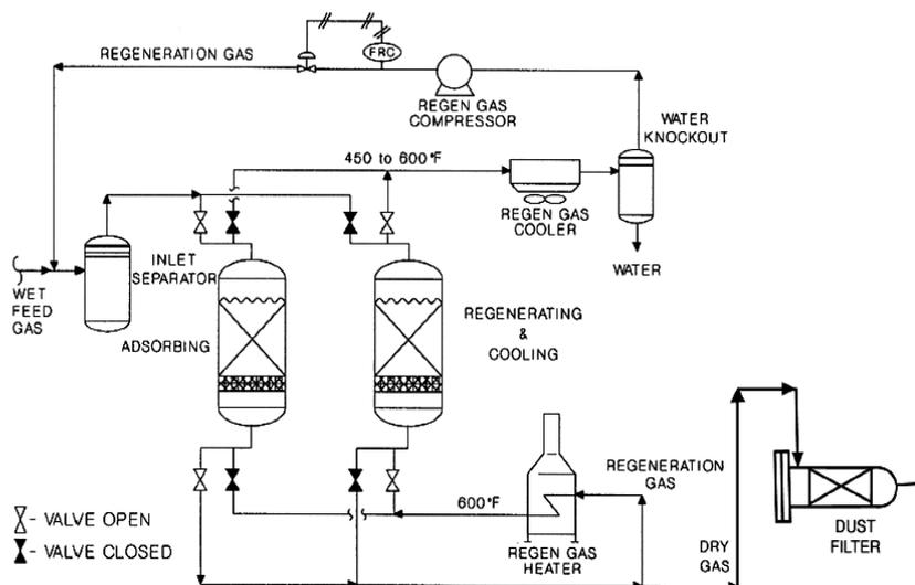
Figure: 3 Basic Flow scheme for solid desiccants
