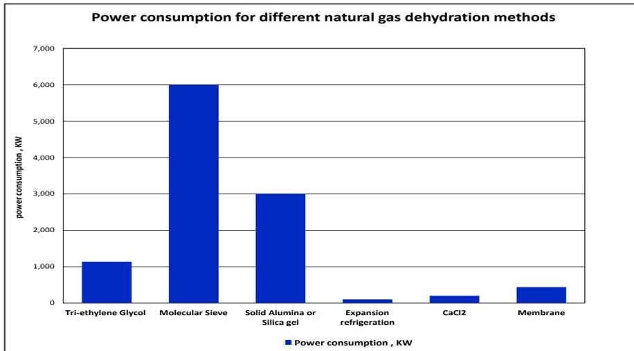
**Figure 7: Power consumption for different natural gas dehydration methods**
