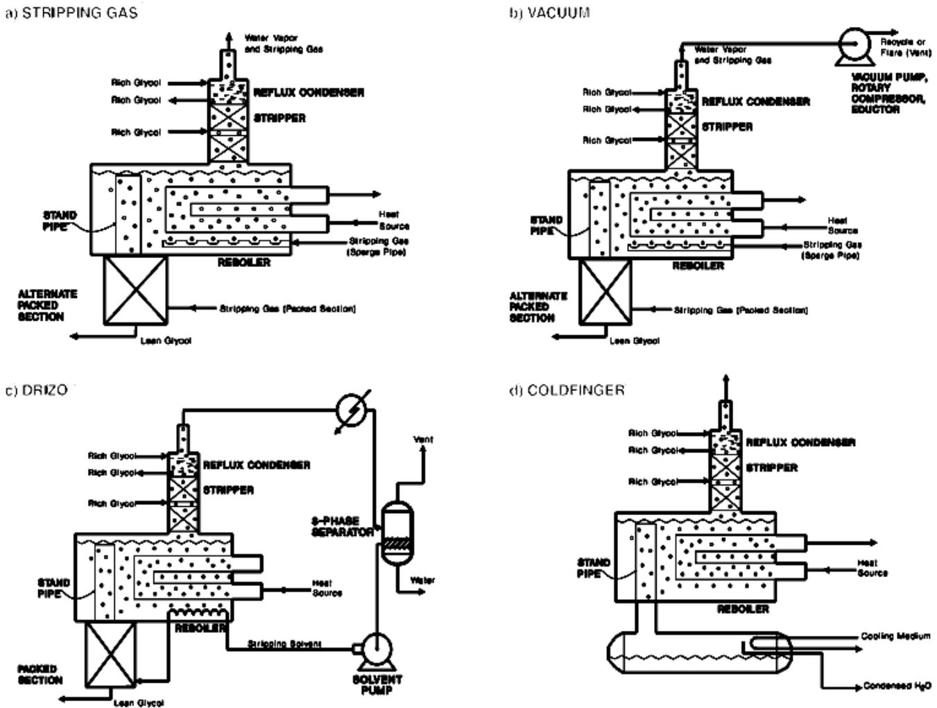
Figure 2 Simplified flow diagram of Enhanced TEG regeneration system
