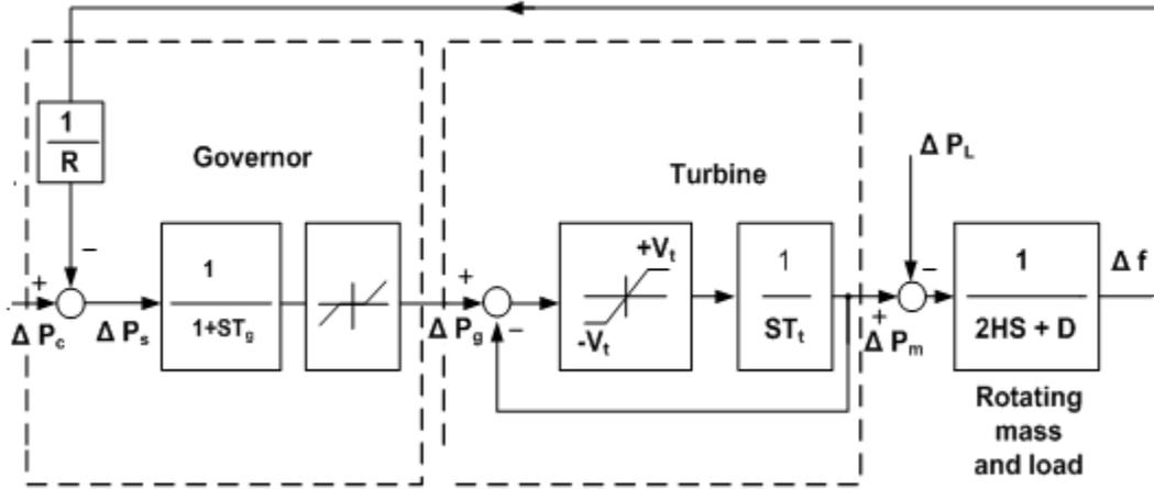
Figure 1. The block diagram of uncontrolled single-area power system.
