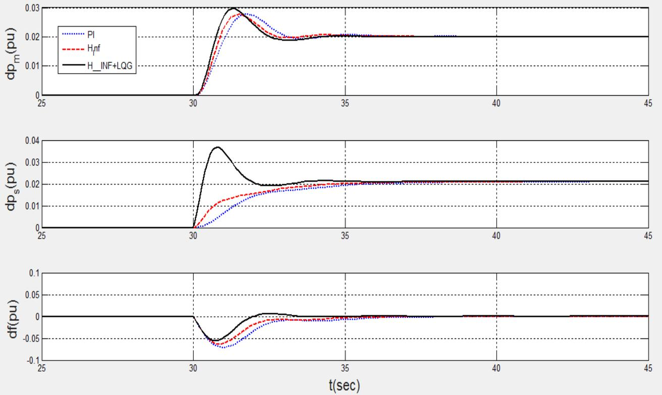
Figure 6: Power system responses to the case 1; a) the governor valve position  $\Delta P_m$ , b) the governor's control signal  $\Delta P_s$ , and c) the frequency deviation  $\Delta f$
