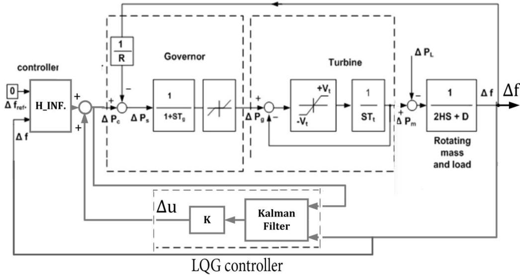
Figure 4: The block diagram of single area power system including the proposed  $H_\infty$ +LQG controllers
