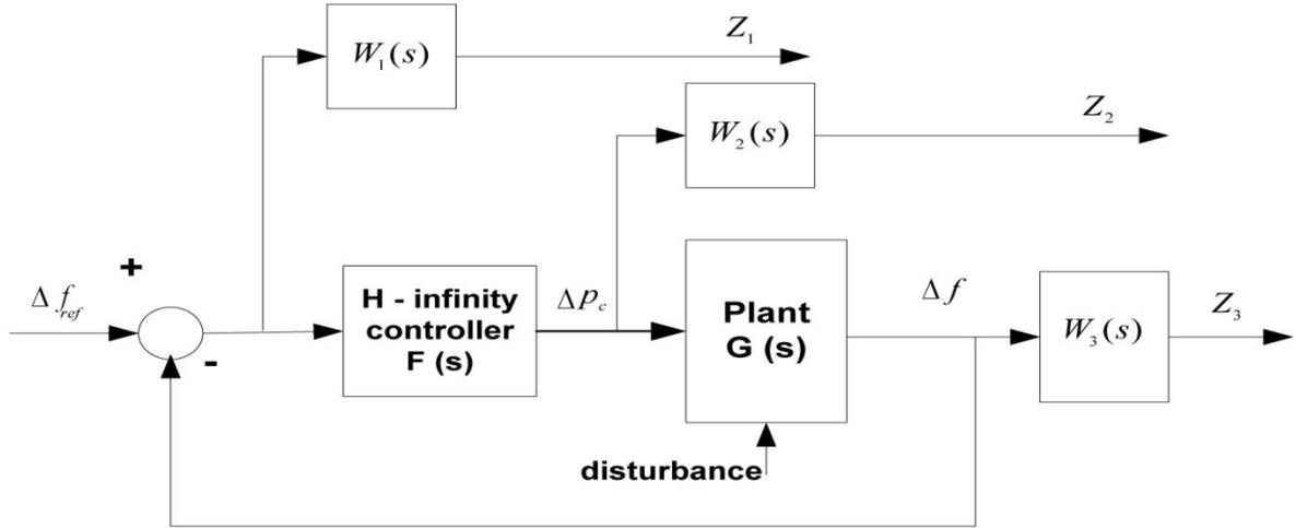
Figure 3: Simplified block diagram of the augmented plant including  $H_\infty$  controller
