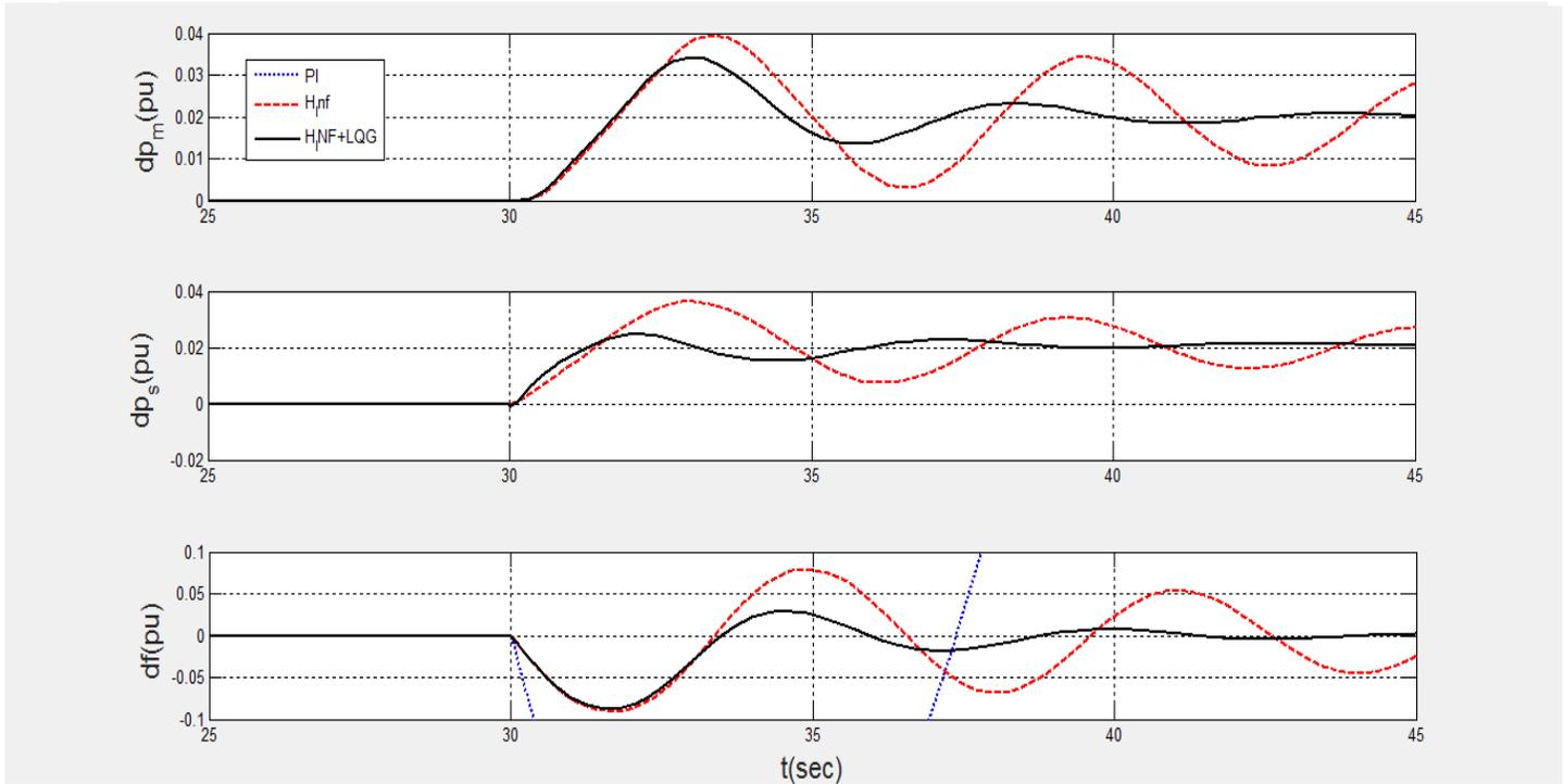
Figure 9: Power system responses to the case 4; a) the governor valve position  $\Delta P_m$ , b) the governor's control signal  $\Delta P_s$ , and c) the frequency deviation  $\Delta f$
