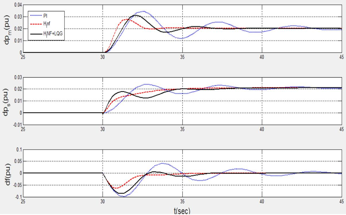
Figure 8: Power system responses to the case 3; a) the governor valve position  $\Delta P_m$ , b) the governor's control signal  $\Delta P_s$ , and c) the frequency deviation  $\Delta f$ , and
