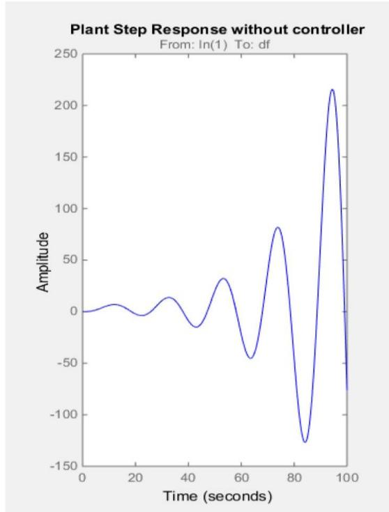
Figure 5. The dynamic performance of the control plant without controller
