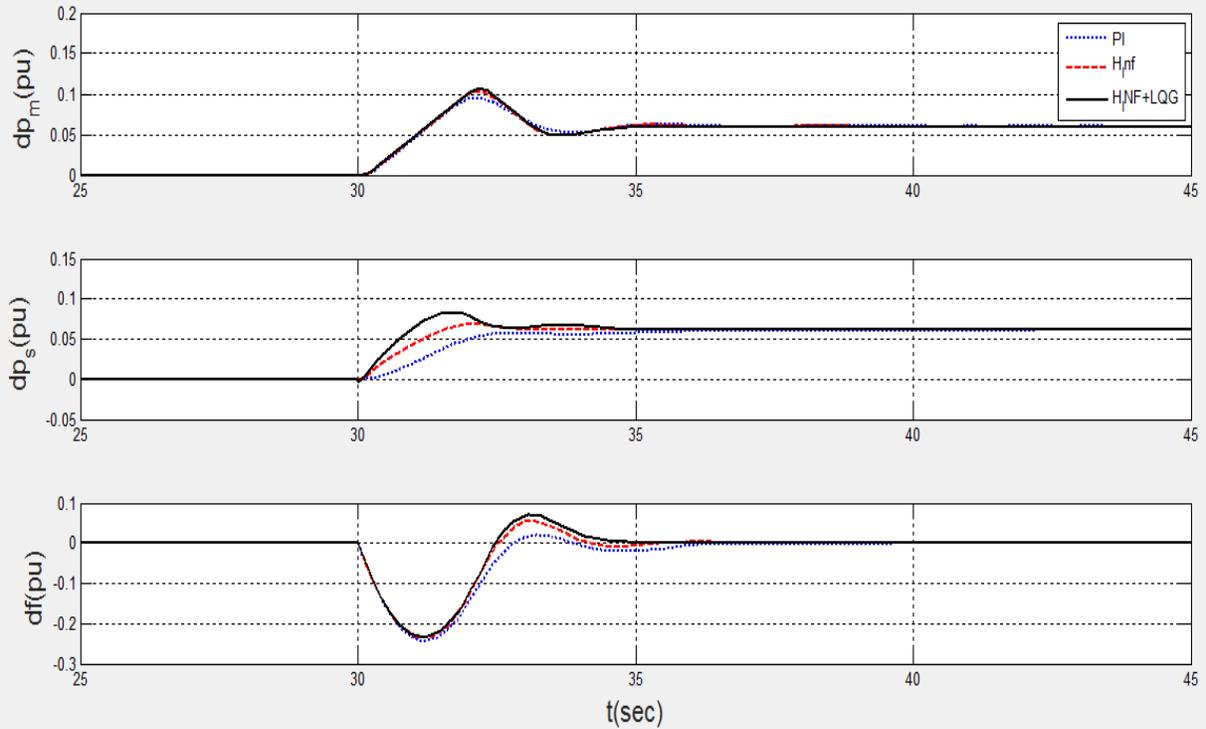
Figure 7: Power system responses to the case 2; a) the governor valve position  $\Delta P_m$ , b) the frequency deviation  $\Delta f$ , and c) the governor's control signal  $\Delta P_s$ .
