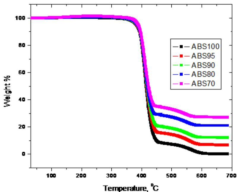
Figure 2 : Thermograms of ABS and ABS/mica composites
