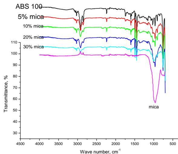
Figure 1 : FTIR spectra of ABS, mica and ABS/mica composites
