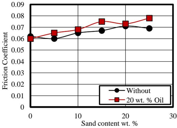
Fig. 3 Friction values caused by rubbing sand against steel surface.
