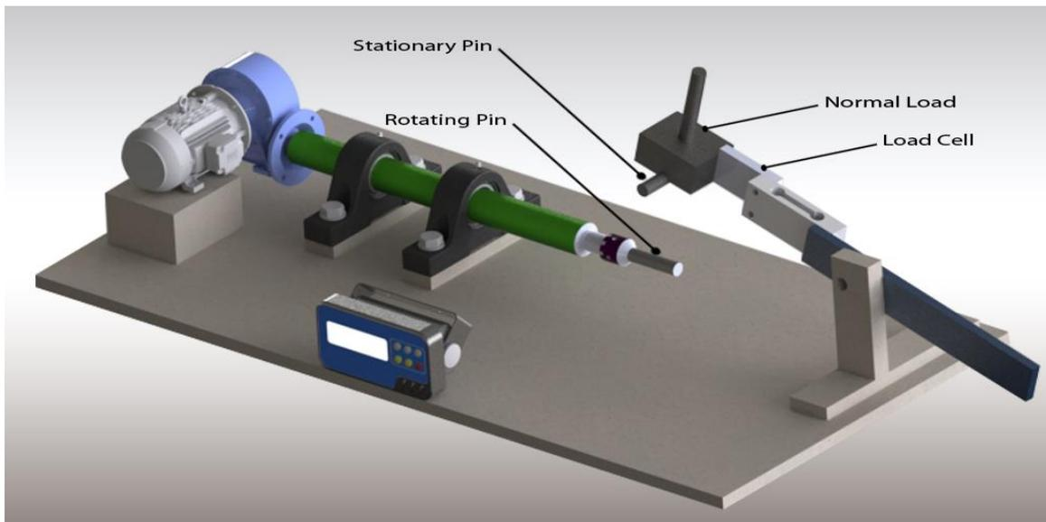
Fig. 1 Layout of cross pin wear tester.
