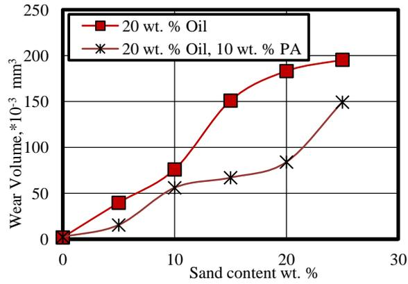
Fig. 9 Effect of adding polyamide to contaminated grease on friction of steel specimen.
