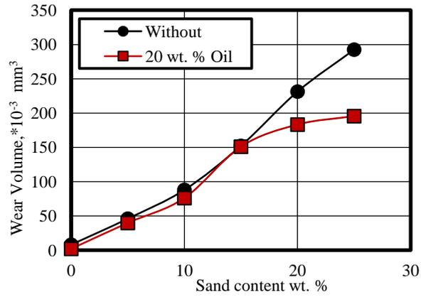
Fig. 4 Wear volume of specimens caused by abrasive sand particles.
