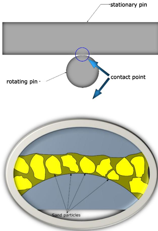
Fig. 5 Effect of abrasive sand particles on friction values.
