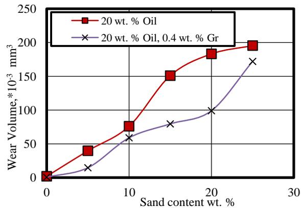
Fig. 7 Effect of sand content contaminating lithium grease.
