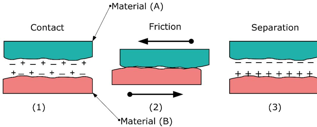
Fig. 12 Tribocharges produced due to rubbing between two different materials.
