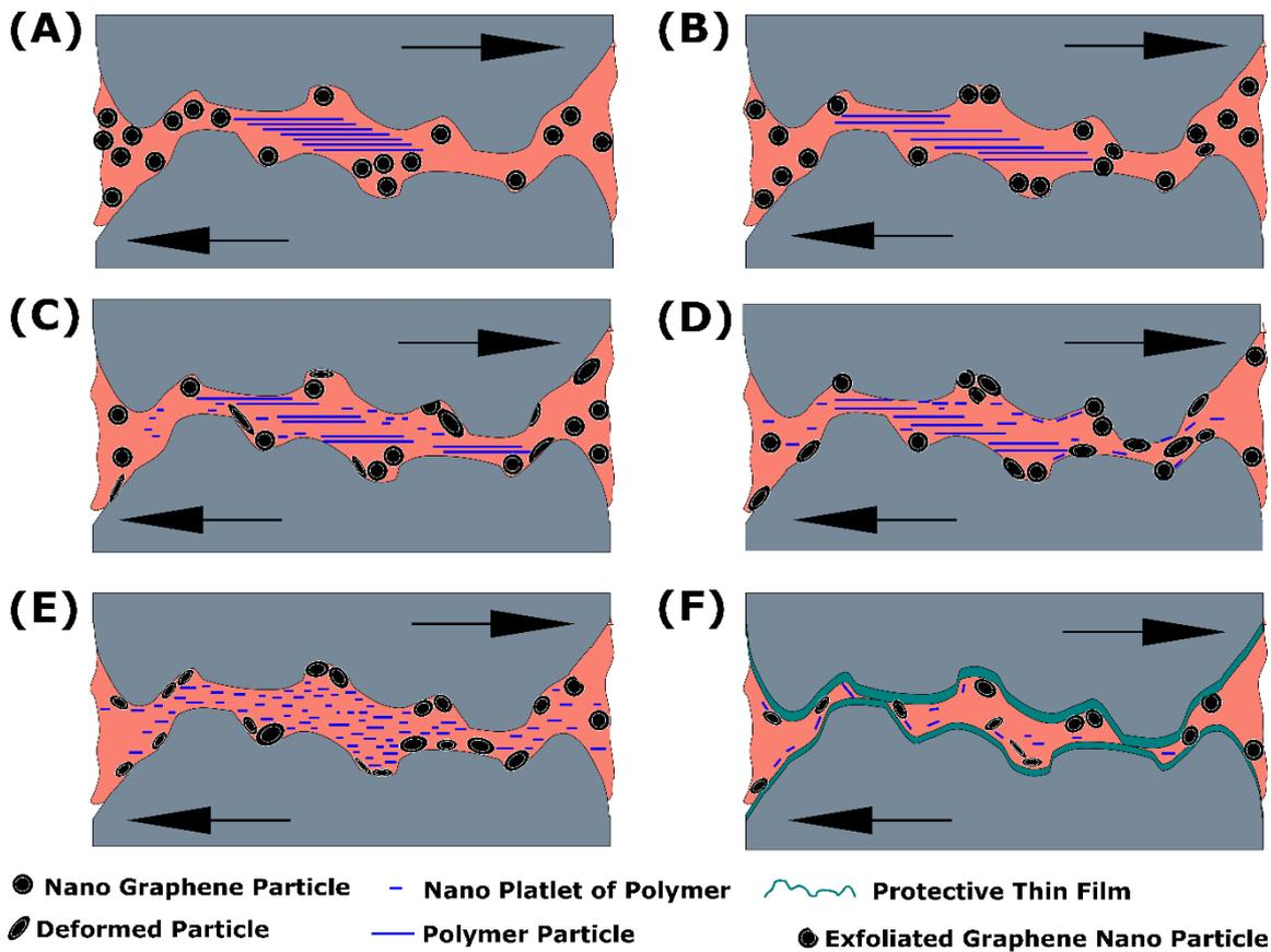
Fig. 15 Effect of polyamide and graphene nano particles on the tribological performance of lithium grease.
