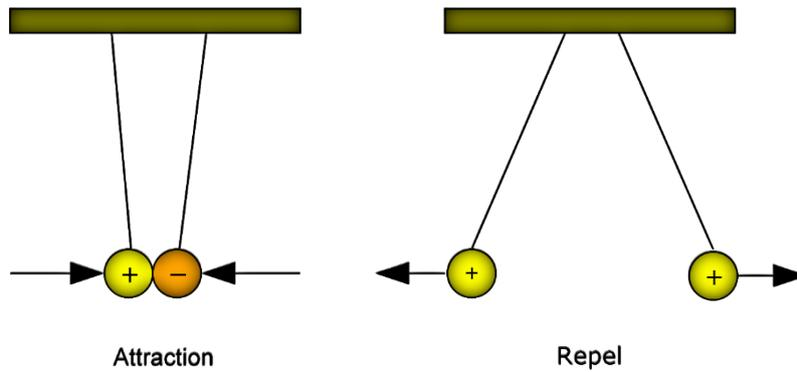
Fig. 11 Similar and dissimilar charges produce due to triboelectrification
