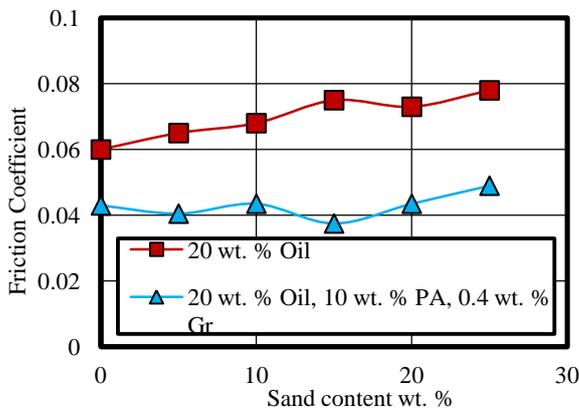
Fig. 13 Effect of PA with nano graphene on friction caused by sand particles.
