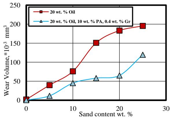
Fig. 14 Wear volume of specimens Caused by abrasive sand particles and method of reducing it.
