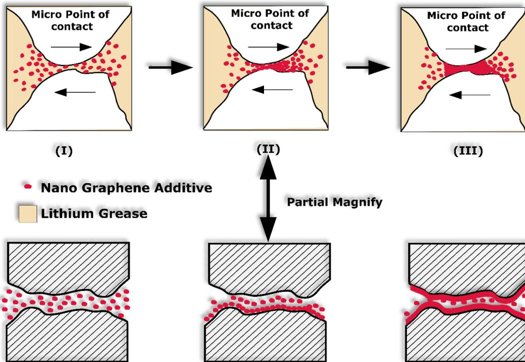
Fig. 8 Schematic sketch of mechanism of 0.4 wt. % of graphene nano particles.
